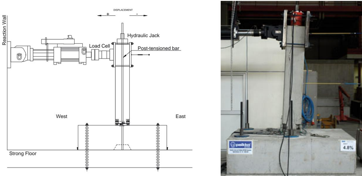
**Fig. 7:** Instrumentation of the connection between column and foundation: (a) side perpendicular to the load direction; (b) side parallel to the load direction.
