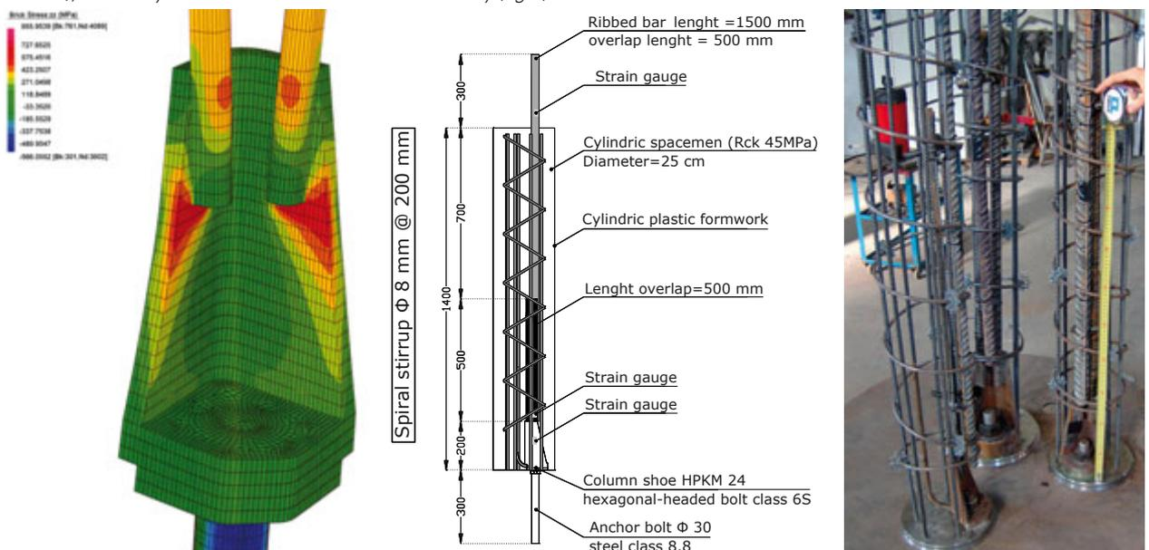
**Tab. 2:** Planning of the tests (3 groups of 4 specimens for each type of column shoe, HPKM 24, 30, 39)
