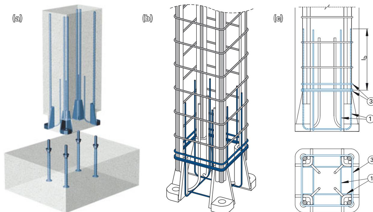
**Fig. 1:** Representation of the studied column to foundation system: a) connection between the shoes and the anchor bolts; b) detail of the welded bars and of the lap splice along the height of the column; c) details of the additional reinforcement
