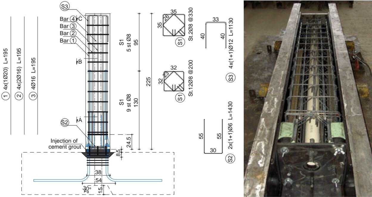
**Fig. 5:** Details of the reinforcement of the connection between column and foundation (4  $\varnothing$ 24mm steel pins added in order to resist shear actions)
