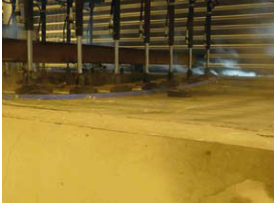
Fig. 8 Deflection of the load distribution plate / transversal deflection of the test panel.
