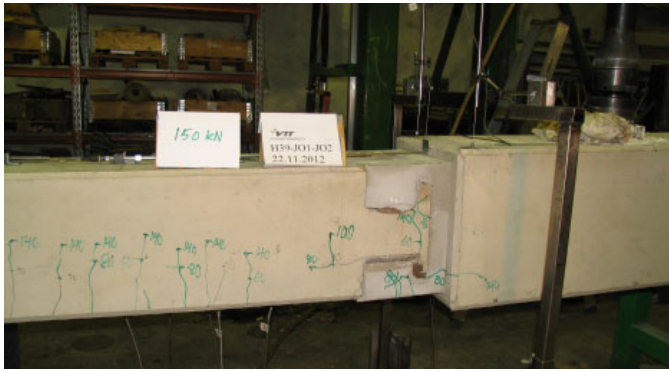
Stiffness test. Note failure in column.
