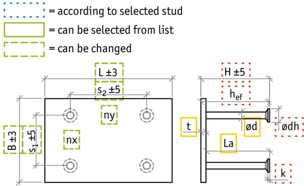
Modified WELDA® Fastening Plates must be named such that they cannot be confused with standard WELDA® Fastening Plates. Manufacturing drawings are required for production. The drawings must show the dimensions of the plate, the sizes and positions of the anchors, and the materials. Contact Peikko's sales team for more information about modifying WELDA® Fastening Plates.
