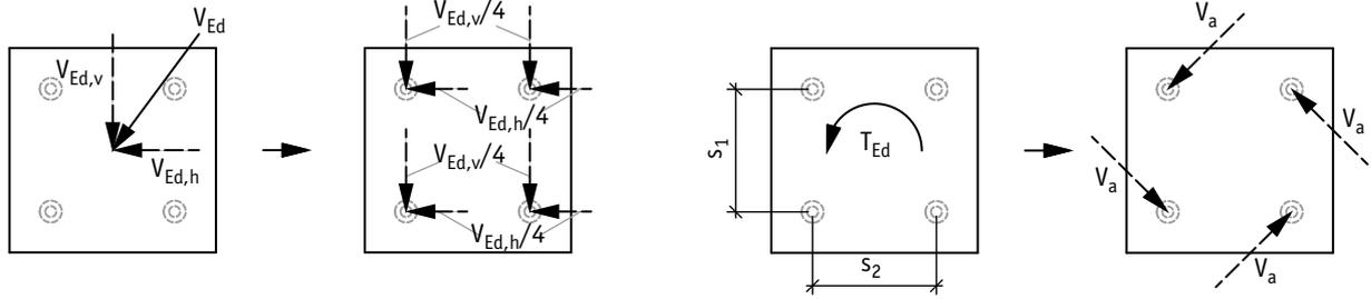
$$V_a = \frac{T_{Ed}}{I_p} \left[ \left( \frac{s_1}{2} \right)^2 + \left( \frac{s_2}{2} \right)^2 \right]^{0.5} \text{ and } I_p = s_1^2 + s_2^2$$
